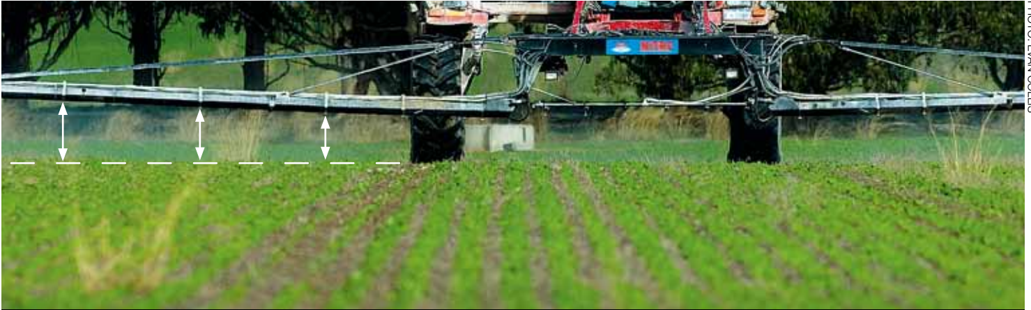
Increasing boom height increases drift risk.
